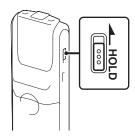
Slide the HOLD switch in the opposite direction from that of the arrow. The IC recorder is turned on, and "ACCESS" flashes.
