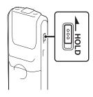
Slide the HOLD switch in the direction of the arrow in the recording or playback mode.
