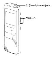
If you connect commercially available headphones to the ∩ (headphone) jack before you start, you can monitor the recording. You can adjust the monitoring volume by pressing VOL +/–, but the recording level is fixed.
