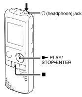
You can record the sound of the IC recorder with other equipment.
