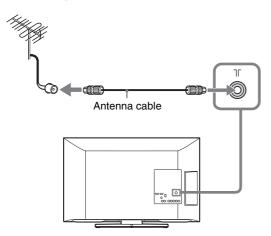
Connecting an antenna/cable and VCR
