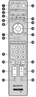
Ϋ́. The number 5, ▶ PROG + and AUDIO buttons have tactile dots. Use the tactile dots as references when operating the TV.
