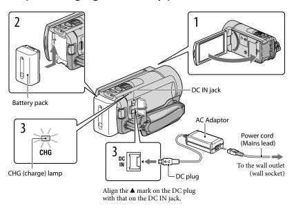
You can charge the "InfoLITHIUM" battery pack (V series) after attaching it to your camcorder.
