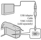
You cannot use the Built-in USB Cable for this type of connection.
