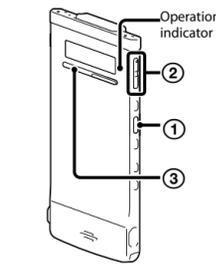
① Press the ENT button. Playback starts and the operation indicator lights in green.
