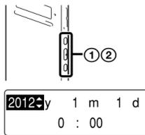
① When the confirmation message for clock setting appears, press the left arrow key or the right arrow key to select "YES," and then press the right arrow key/ENT.
