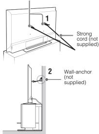
\* KLV-40EX430, KLV-40EX43A, KLV-40EX43B: Use M6 anchor bolts KLV-32EX330, KLV-32EX33A, KLV-32EX33B: Use M4 anchor bolts
