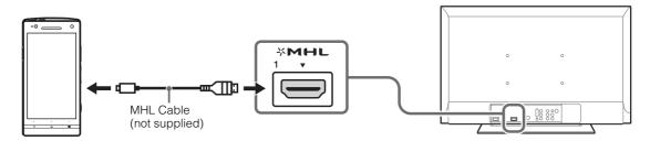
The MHL (Mobile High-Definition Link) enables the TV to communicate with connected MHL-compatible device. When connecting MHL-compatible device, TV simultaneously charges the connected device while playing photo/music/video from it. You can use the TV remote control to control the connected MHL-compatible device.
