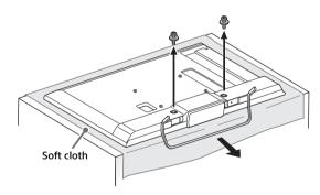
1 Remove the screws from the rear of the TV.
