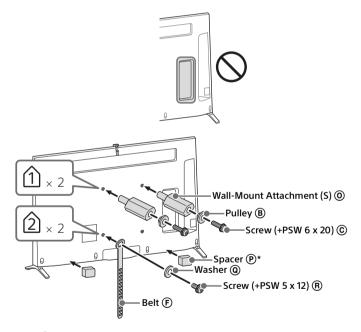
\* Attach Spacer (P) on the flat area of the bottom edge after peeling the separator.
