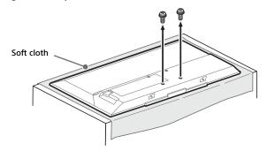
3 Attach the Attachment parts for Wall-Mount Bracket. Check the Attachment parts by referring to "1" of the Wall-Mount Bracket Installation Guide.
